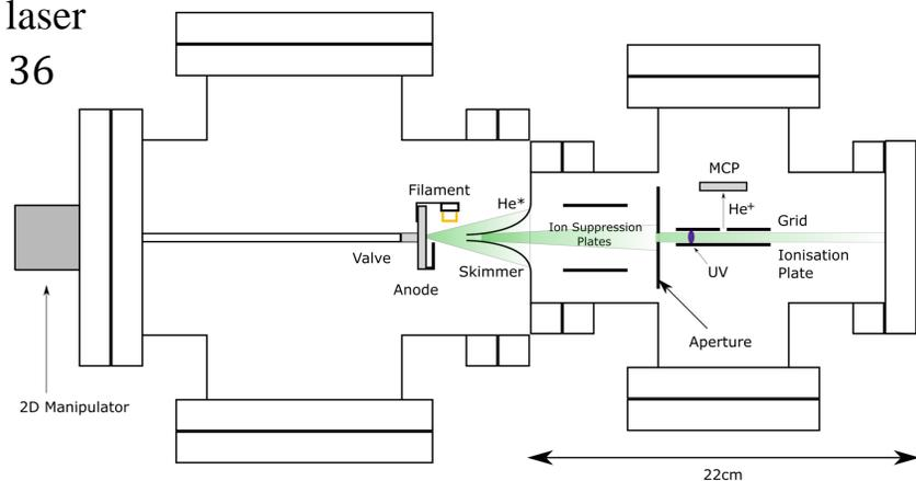
Fig. 1: Schematic of current experimental apparatus.
