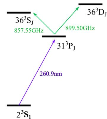
Fig. 2: Energy-level diagram showing possible single-colour single-photon excitation pathways.
