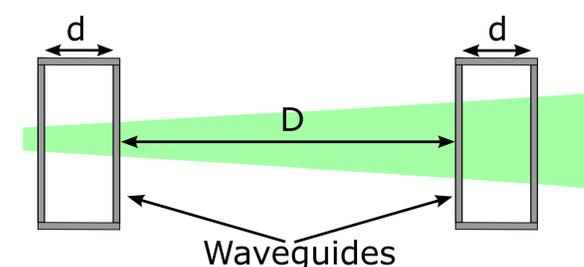
Fig. 8: Example configuration for spatially separated oscillatory field measurements where the green cone indicates a beam of atoms, and the grey boxes are identical microwave guides.
