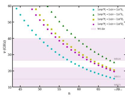
Fig. 6: Targetable single-photon microwave transitions.
