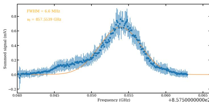
Fig. 9: Measured THz linewidth for  $n=31$  to  $n=36$  transition.
