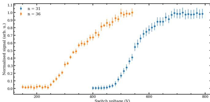
Fig. 4: State-selective field ionization for  $n=31$  and  $n=36$ .
